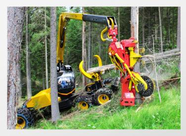
an enourmous terrain flexibility due to the syncronised step and drive movement.
